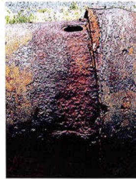
Evidence of pipe failure and exterior corrosion.
