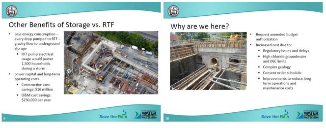
Receiving end of storag facility shown in middle of picture - large box 50 ft. down, will hold pumps; bldg on top shown in later picture; blue and red pipes just supports for open cut, removed once tunnels were built, now all covered, will be part of parking lot
